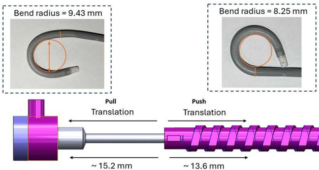
Fig. 2. Push-pull motion and the respective maximum displacement and bending radius of the designed ultra-steerable catheter.
