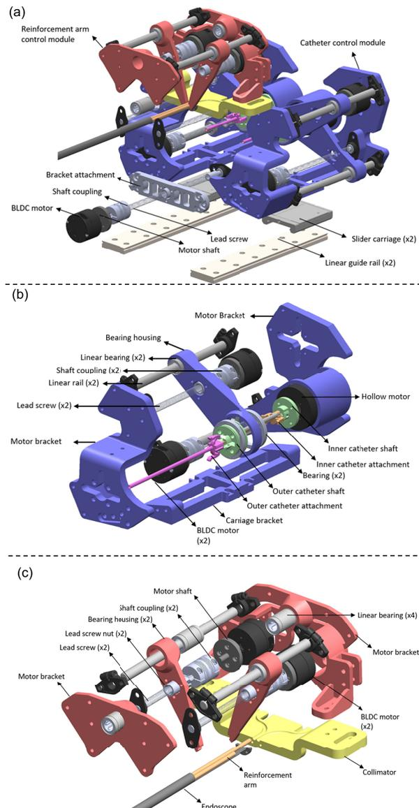
Fig. 1. (a) overview of the CAD model neurosurgery robot, which also depicts the overall modular assembly. (b) design of ultra-steerable catheter control module. (c) design of working channel tube control module
